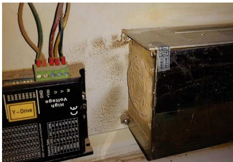
Not only will this cause overheating and thus eventually destroy the power supply, it is also a huge fire danger.
