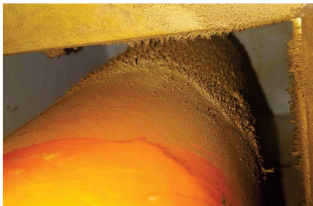
This tube's life was greatly reduced, costing the owner a lot to replace. Keeping it clean would have helped.
