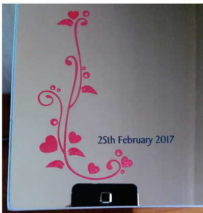
Mirror reverse-engraved and filled from the back with acrylic paint - note the phone camera reflection.
