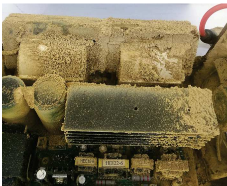
Wood dust is highly combustible, and will also cause the high voltage to arc - recipe for disaster.
