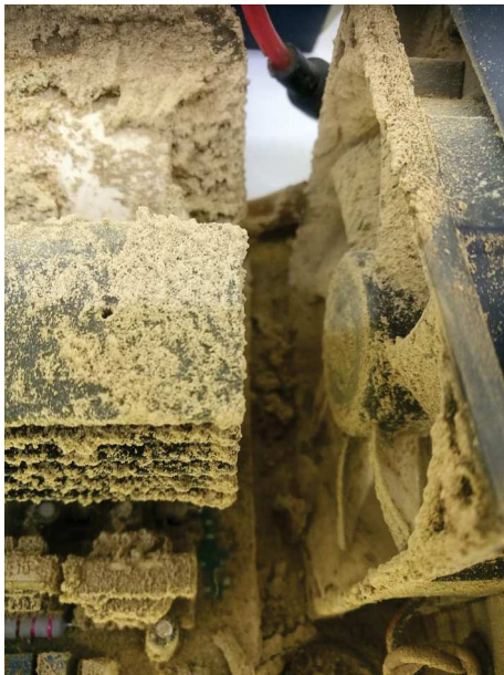
Filthy dirty, icky, clogged, and downright dangerous. This is a fire waiting to happen
