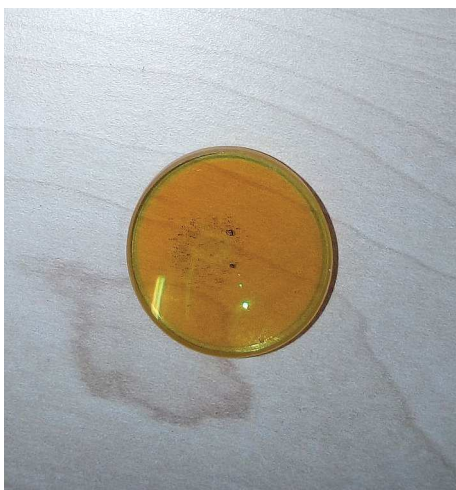
Dust spots burned into the lens will cause the beam not to focus correctly - new lens needed.
