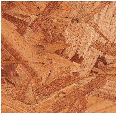
This is OSB (Oriented Strand Board) - not plywood
