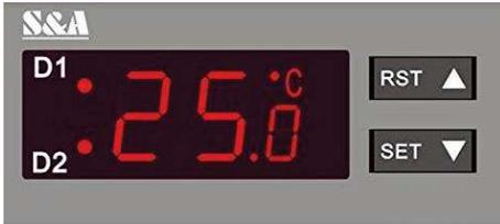
The default control panel showing that D1 is on, meaning it is in "Intelligent Control Mode".
