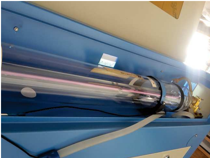
The laser beam firing in the tube. This is for us to check the colour of the beam, which should be bright pink.
